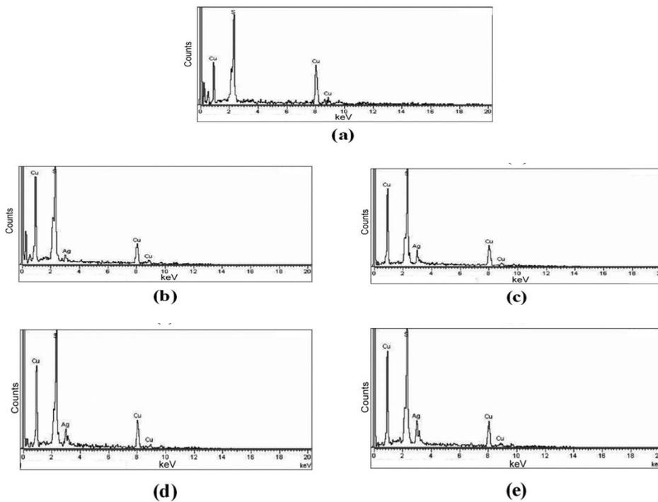
**Fig.5 EDS spectra of (0.05mM) SDBS assisted CuS doped with Ag: (a) 0.0 (b) 0.05 mM, (c) 0.1 mM, (d) 0.15 mM and (e) 0.2 mM**
