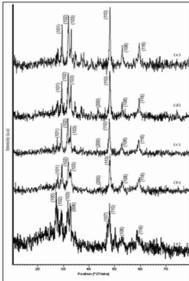
**Fig 1. XRD patterns of (0.05mM) SDBS assisted CuS doped with Ag: (a) 0.0, (b) 0.05 mM, (c) 0.1 mM, (d) 0.15 mM and (e) 0.2 mM**
