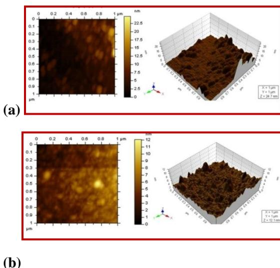
**Fig.6 AFM images of of Ag doped SDBS assisted CuS 0.05 and (b) 0.10 mM**
