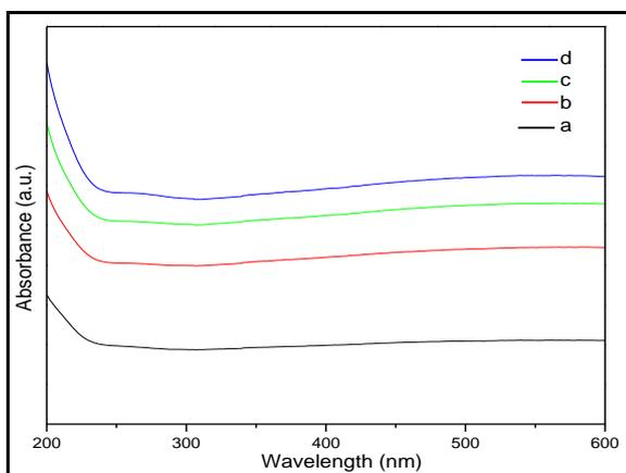
**Fig.2 UV- Visible absorption spectra of Ag doped SDBS assisted CuS (a) 0.05 mM, (b) 0.1 mM, (c) 0.15 mM and (d) 0.2 mM**
