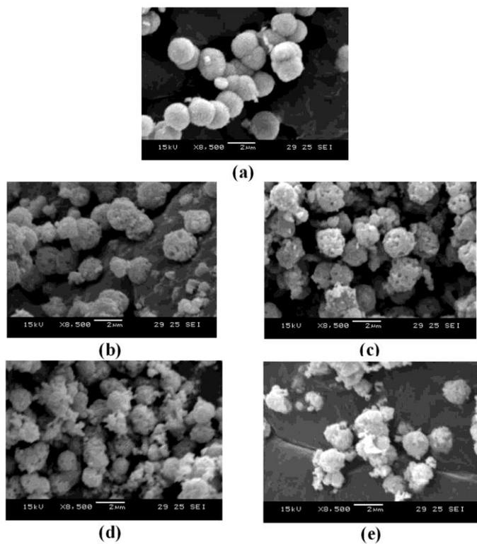
**Fig.4** SEM Photographs of (0.05mM) SDBS assisted CuS doped with Ag: (a) 0.0 (b) 0.05 mM, (c) 0.1 mM, (d) 0.15 mM and (e) 0.2 mM
